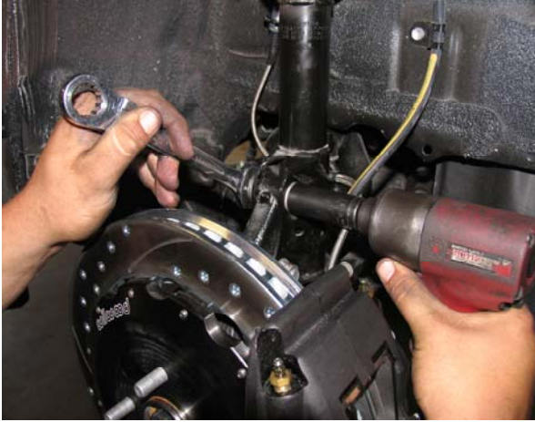
Remove stock strut
