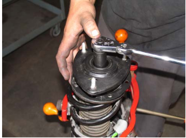
Compress spring and remove hat
