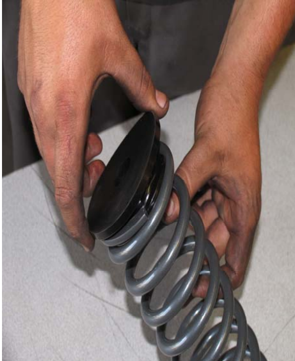
Thread bump stop / isolator onto spring
